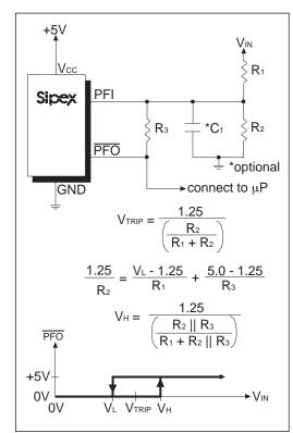
Figure 18. Adding Hysteresis to the POWER-FAIL Comparator
