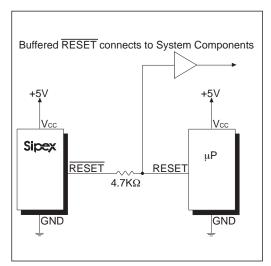
Figure 20. Interfacing to Microprocessors with Bidirectional RESET I/O
