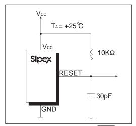
Figure 5B. Circuit for the SP690A/802L  $\overline{RESET}$  Response Time
