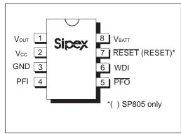
Figure 10. Pinout
