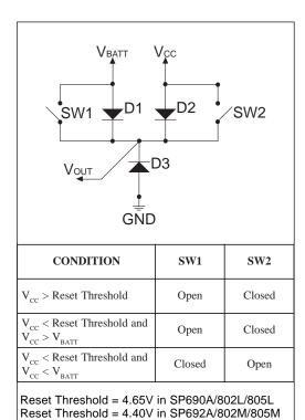
Figure 13. BACKUP-BATTERY Switchover Block Diagram
