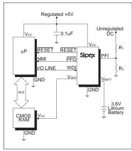
Figure 12. Typical Operating Circuit
