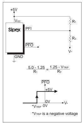
Figure 19. Monitoring a Negative Voltage
