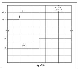
Figure 8A. Power-Fail Comparator Response Time (RISE)
