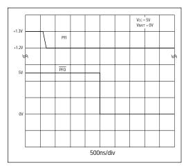
Figure 7A. Power-Fail Comparator Response Time (FALL)
