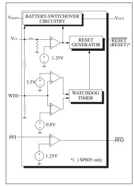
Figure 11. Internal Block Diagram
