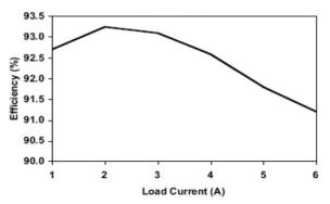
Fig. 5: Efficiency versus Output Current  $V_{\text{IN}}$ =5V,  $V_{\text{OUT}}$ =3.3V
