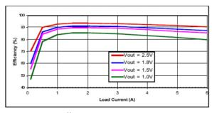
Fig. 11: Efficiency versus Output Current  $V_{\text{IN}}$ =3.3V
