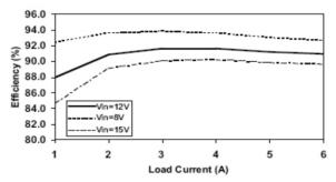
Fig. 3: Efficiency versus Output Current  $V_{\text{IN}}$ =8V, 12V and 15V,  $V_{\text{OUT}}$ =5V
