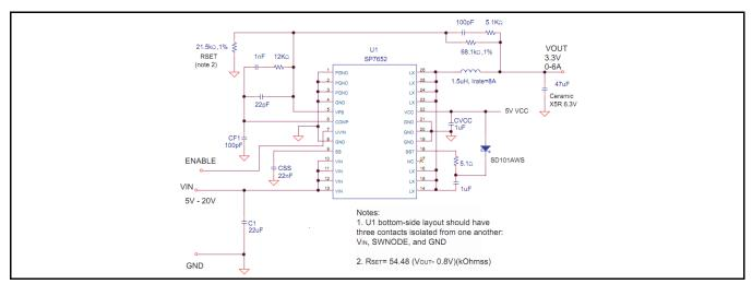
Fig. 1: SP7652 Application Diagram
