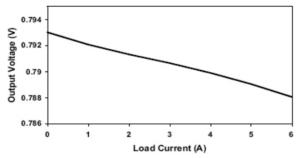
Fig. 8: Output Voltage versus Output Current  $V_{IN}=3.3V$ ,  $V_{OUT}=0.8V$
