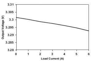
Fig. 6: Output Voltage versus Output Current  $V_{\text{IN}}$ =5V,  $V_{\text{OUT}}$ =3.3V
