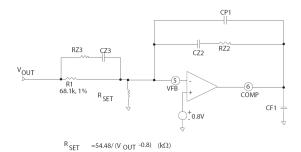
Fig. 14: Type III Error Amplifier Compensation Circuit
