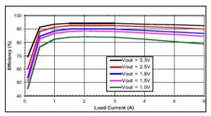
Fig. 10: Efficiency versus Output Current  $V_{\text{IN}}$ =5V
