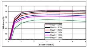
Fig. 9: Efficiency versus Output Current  $V_{\text{IN}} {=}\, 12 V$
