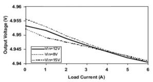
Fig. 4: Output Voltage versus Output Current  $V_{\text{IN}}{=}8V$ , 12V and 15V
