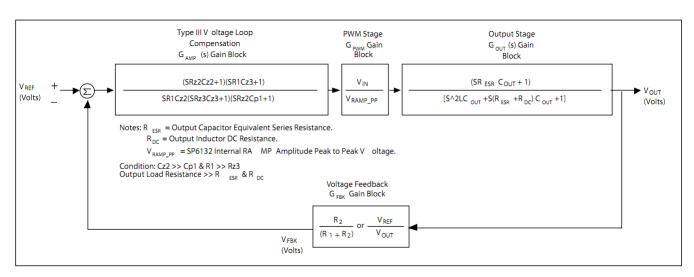
Fig. 12: SP7652 Voltage Mode Control Loop
