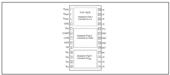
Fig. 2: SP7652 Pin Assignment
