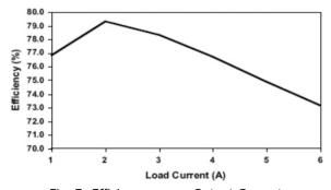
Fig. 7: Efficiency versus Output Current  $V_{\text{IN}}{=}3.3\text{V},\,V_{\text{OUT}}{=}0.8\text{V}$
