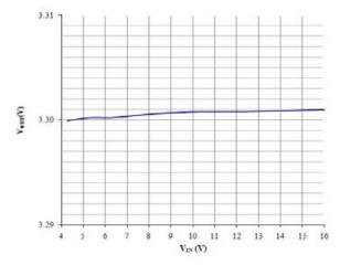
Figure 6: Line Regulation: I<sub>OUT</sub> = 10mA, V<sub>OUT</sub> = 3.3V
