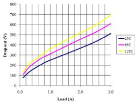
Figure 4: Dropout Voltage vs. Load Current
