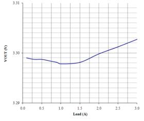
Figure 7: Load Regulation: V<sub>OUT</sub> = 3.3V
