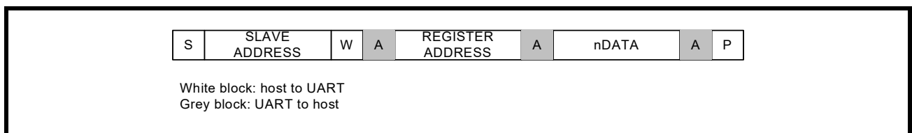
FIGURE 4. MASTER WRITES TO SLAVE (XR20M1170)
