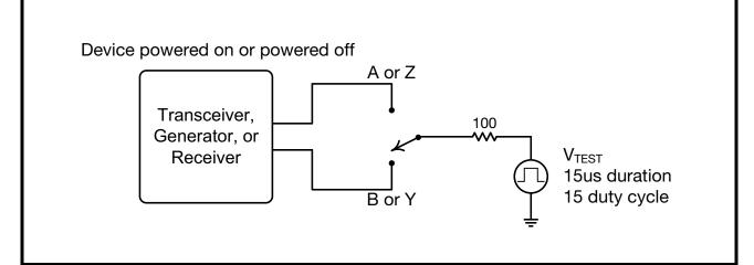
FIGURE 6. DRIVER PROPAGATION DELAY TEST CIRCUIT & TIMING DIAGRAM
