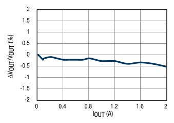
Figure 7. Load Regulation Channel 3, 5V<sub>IN</sub>, 1.2V<sub>OUT</sub>
