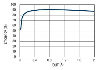
Figure 14. Efficiency Channel 1, 12V<sub>IN</sub> 3.3V<sub>OUT</sub>
