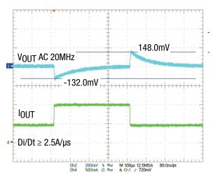
Figure 10. 12V<sub>IN</sub>, 3.3V<sub>OUT</sub> Transient Response, 0.5A to 1.0A
