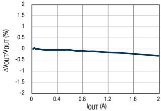
Figure 3. Load Regulation Channel 1,  $5V_{IN}$ , 3.3 $V_{OUT}$
