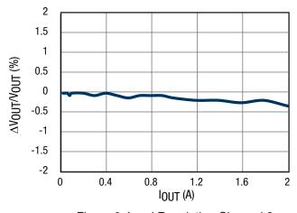
Figure 6. Load Regulation Channel 3, 12V<sub>IN</sub>, 1.2V<sub>OUT</sub>
