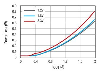
Figure 23. Channel 3 Power Loss at  $f_{SW} = 500kHz$ ,  $V_{IN} = 12V$ , No Airflow
