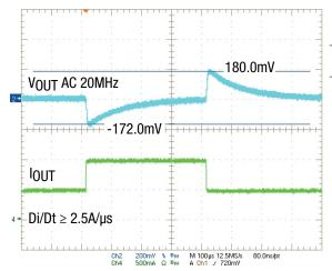
Figure 9. 12V<sub>IN</sub>, 5.0V<sub>OUT</sub> Transient Response, 0.5A to 1.0A
