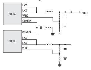
Figure 31. Parallel Operation
