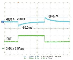
Figure 13. 5V<sub>IN</sub>, 1.8V<sub>OUT</sub> Transient Response, 0.5A to 1.0A
