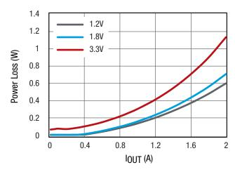
Figure 24. Channel 1 Power Loss at  $f_{SW} = 500kHz$ ,  $V_{IN} = 5V$ , No Airflow
