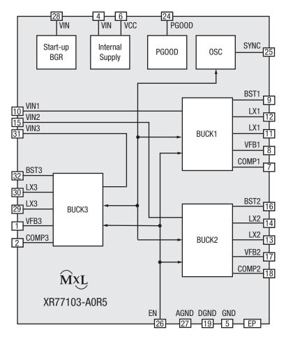
Figure 27. Functional Block Diagram
