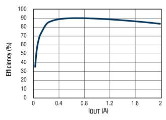
Figure 15. Efficiency Channel 1, 5V<sub>IN</sub> 3.3V<sub>OUT</sub>
