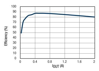
Figure 16. Efficiency Channel 2, 12V<sub>IN</sub> 1.8V<sub>OUT</sub>
