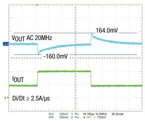
Figure 12. 5V<sub>IN</sub>, 3.3V<sub>OUT</sub> Transient Response, 0.5A to 1.0A
