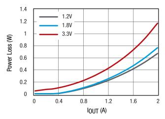
Figure 26. Channel 3 Power Loss at  $f_{SW} = 500 kHz$ ,  $V_{IN} = 5V$ , No Airflow
