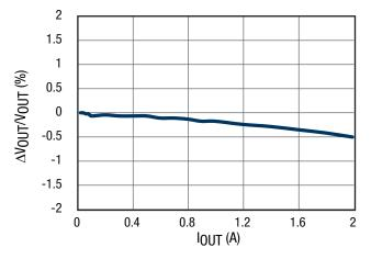
Figure 2. Load Regulation Channel 1, 12V<sub>IN</sub>, 3.3V<sub>OUT</sub>
