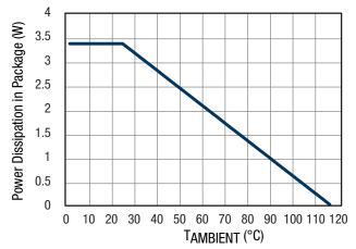
Figure 20. Package Thermal Derating
