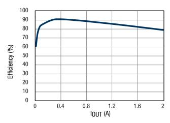
Figure 17. Efficiency Channel 2, 5V<sub>IN</sub> 1.8V<sub>OUT</sub>
