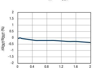
Figure 4. Load Regulation Channel 2, 12V<sub>IN</sub>, 1.8V<sub>OUT</sub>
