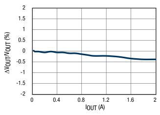
Figure 5. Load Regulation Channel 2, 5V<sub>IN</sub>, 1.8V<sub>OUT</sub>
