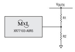
Figure 28. Output Voltage Setting
