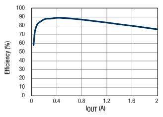
Figure 19. Efficiency Channel 3,  $5V_{IN}$  1.2 $V_{OUT}$
