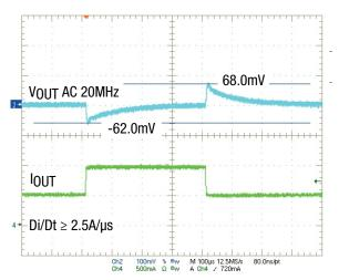
Figure 11. 12V<sub>IN</sub>, 1.8V<sub>OUT</sub> Transient Response, 0.5A to 1.0A
