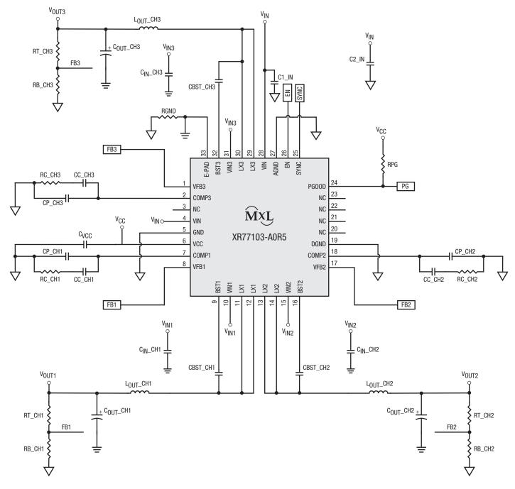
Figure 32. Typical Applications Schematic
