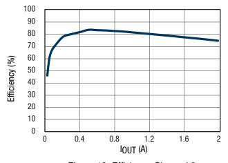
Figure 18. Efficiency Channel 3, 12V<sub>IN</sub> 1.2V<sub>OUT</sub>
