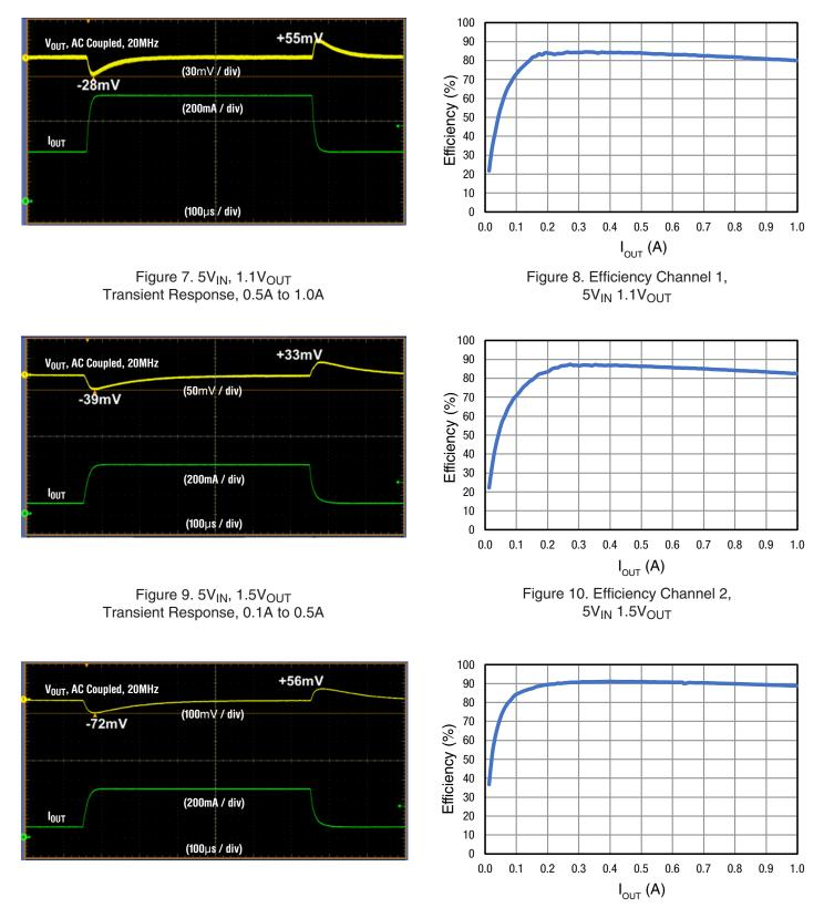
Figure 11.  $5V_{\text{IN}},\,3.3V_{\text{OUT}}$  Transient Response, 0.1A to 0.5A
