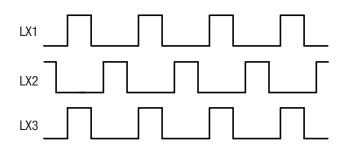
Figure 28. Out-of-Phase Operation
