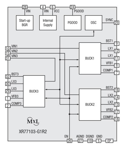
Figure 27. Functional Block Diagram
