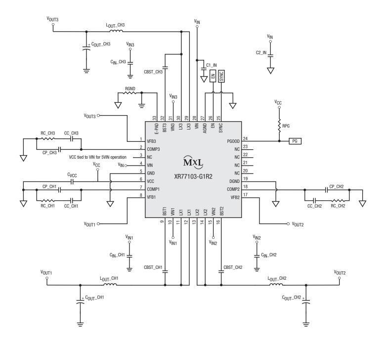
Figure 30. Typical Applications Schematic
