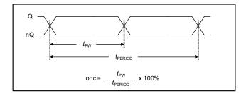
Figure 10: Output Period and Duty Cycle
