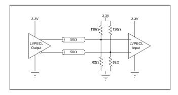
Figure 5: XR81111 3.3V LVPECL Output Termination
