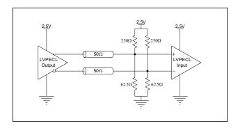
Figure 6: XR81111 2.5V LVPECL Output Termination
