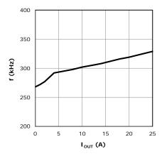
Fig. 22: frequency versu IOUT, Forced CCM
