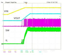
Fig. 9: Powerup, Forced CCM, I<sub>OUT</sub> = 25A
