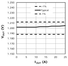
Fig. 4: Load regulation,  $V_{IN} = 12V$
