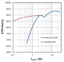
Fig. 15: Efficiency, 12VIN, 3.3VOUT, 1uH, 300kHz
