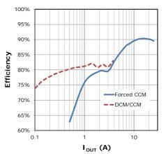
Fig. 17: Efficiency, 12VIN, 1.8VOUT, 1uH, 300kHz
