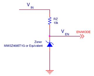
Figure 29. Selecting DCM/CCM by deriving EN/MODE from  $V_{\text{IN}}$
