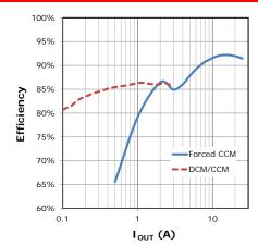
Fig. 16: Efficiency,  $12V_{IN}$ ,  $2.5V_{OUT}$ , 1uH, 300kHz
