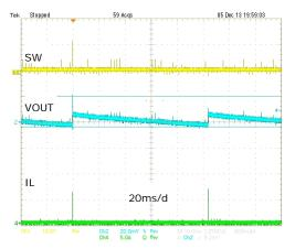
Fig. 7:  $V_{\text{OUT}}$  ripple is 22mV at OA, DCM, 12V<sub>IN</sub>, 1.2V<sub>OUT</sub>
