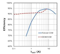
Fig. 12: Efficiency,  $5V_{IN}$ ,  $1.8V_{OUT}$ , 0.47uH, 300kHz
