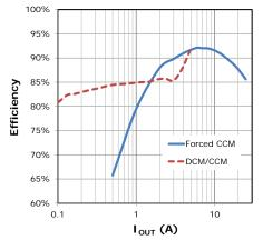
Fig. 14: Efficiency, 5VIN, 1.0VOUT, 0.47uH, 300kHz
