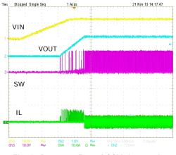
Fig. 8: Powerup, Forced CCM,  $I_{OUT} = OA$
