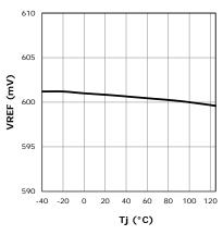
Fig. 23: VREF versus temperature
