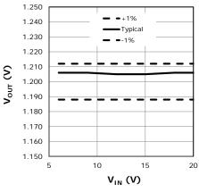
Fig. 5: Line regulation,  $I_{OUT} = 25A$
