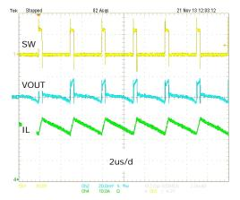
Fig. 6: Vout ripple is 22mV at 25A, 12VIN, 1.2VOUT
