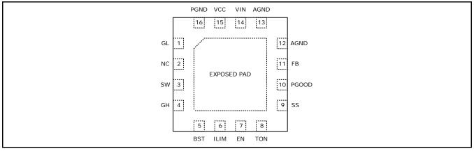
Fig. 3: XRP6141 Pin Assignment
