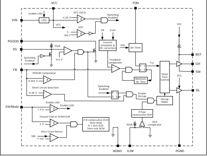
Fig. 2: XRP6141 Block Diagram
