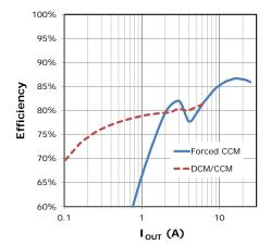
Fig. 18: Efficiency,  $12V_{IN}$ ,  $1.2V_{OUT}$ , 0.47uH, 300kHz
