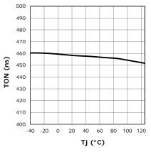
Fig. 24: On-Time versus temperature
