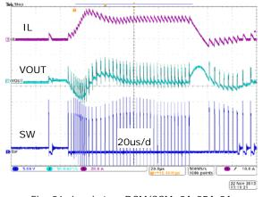
Fig. 26: Load step, DCM/CCM, 0A-25A-0A
