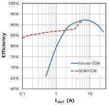
Fig. 13: Efficiency, 5V<sub>IN</sub>, 1.2V<sub>OUT</sub>, 0.47uH, 300kHz
