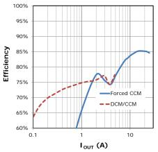
Fig. 19: Efficiency, 12VIN, 1.0VOUT, 0.47uH, 300kHz
