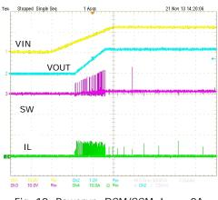
Fig. 10: Powerup, DCM/CCM,  $I_{OUT} = 0A$
