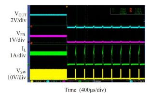
Fig. 14: Onset of Short-circuit Protection  $I_{\text{OUT}}$ =1.5A
