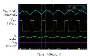
Fig. 10: Output Ripple at  $I_{OUT}=1.5A$
