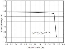
Fig. 7: Output Voltage versus Output Current
