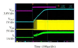
Fig. 12: Enable Turn-on Characteristic  $2.6\Omega$  resistive Load
