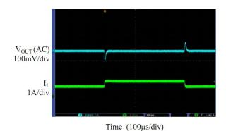
Fig. 11: Load Step Transient,  $I_{\text{OUT}}$ =1A to 1.5A
