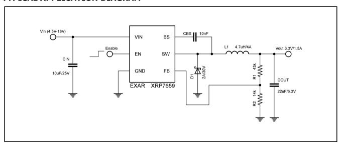
Fig. 1: XRP7659 Application Diagram
