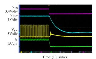
Fig. 13: Enable Turn-off Characteristic  $2.6\Omega$  resistive Load
