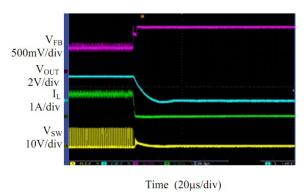
Fig. 16: Onset of Over-voltage Protection,  $I_{OUT}=1.5A$
