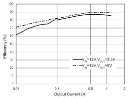
Fig. 4: Efficiency versus Output Current, V<sub>IN</sub>=12V
