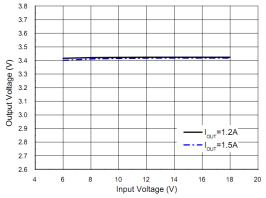
Fig. 8: Output Voltage versus Input Voltage
