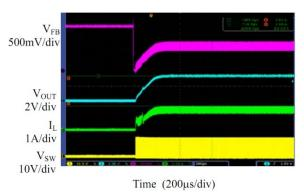
Fig. 17: Over-voltage Recovery, I<sub>OUT</sub>=1.5A
