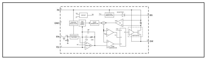
Fig. 2: XRP7659 Block Diagram
