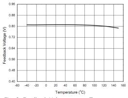
Fig. 6: Feedback Voltage versus Temperature
