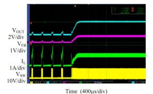
Fig. 15: Short-circuit recovery  $R_{LOAD}=2.6\Omega$
