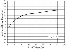
Fig. 9: Maximum Output Current versus Input Voltage
