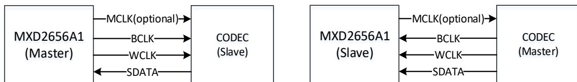
Figure 36 I2S interface signals
