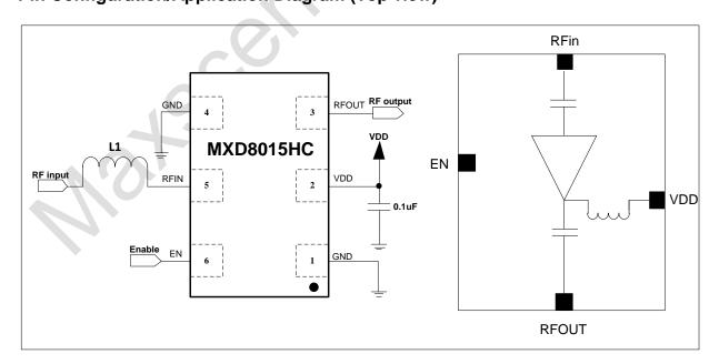
Figure 1 MXD8015HC application circuit
