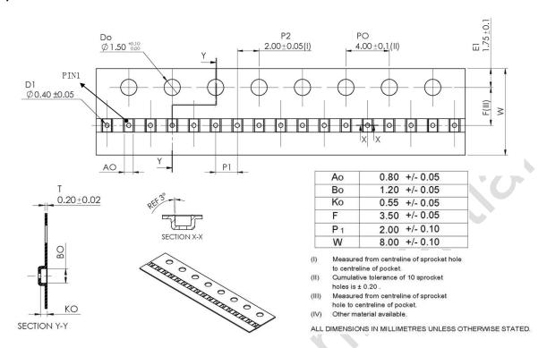
Figure 4 Tape and reel dimensions
