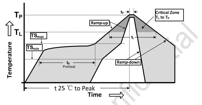
Figure 5. Recommended Lead-Free Reflow Profile
