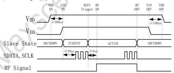
Note: VIO can be applied to the device before VDD or removed after VDD.
