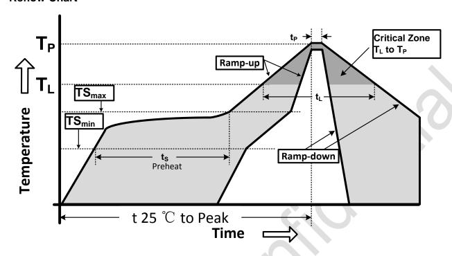
Figure 7. Recommended Lead-Free Reflow Profile
