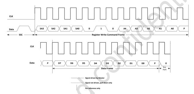
Figure 3. Register Write Command Sequence
