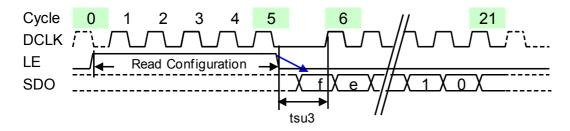
"Read configuration" command is used to read the configuration register of MBI5252. When this command is received, the 16-bit data of configuration register will be shifted out from SDO pin, as shown in the above waveform, and MSB bit will be shifted out first.
