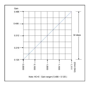
The 6 bits (bit 5~bit 0) of the configuration register set the gain of output current, i.e., G. As total 6-bit in number, i.e., ranging from 6'b000000 to 6'b111111, these bits allow user to set the output current gain up to 64 levels. These bits can be further defined inside configuration register as follows:
