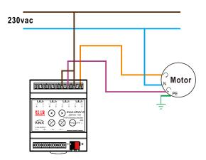
Note: Check installation manual of shutter motor for wiring.
