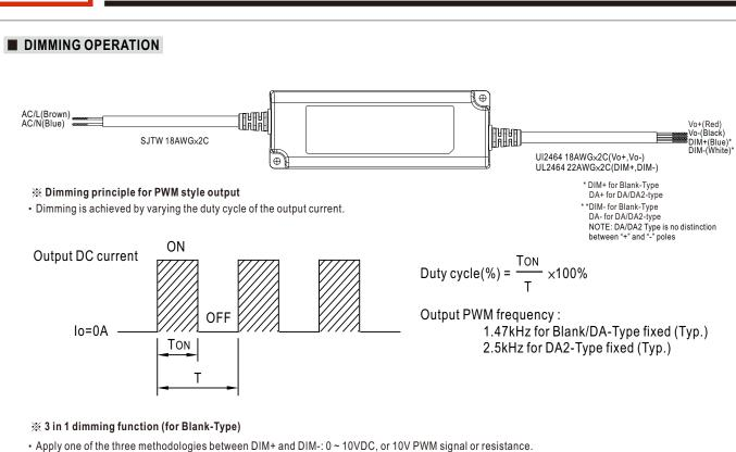
• Dimming source current from power supply:  $100\mu A$  (typ.)
