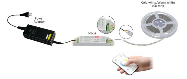
Note: Connection according to the strip with the actual definition of location wiring, line color only for reference.
