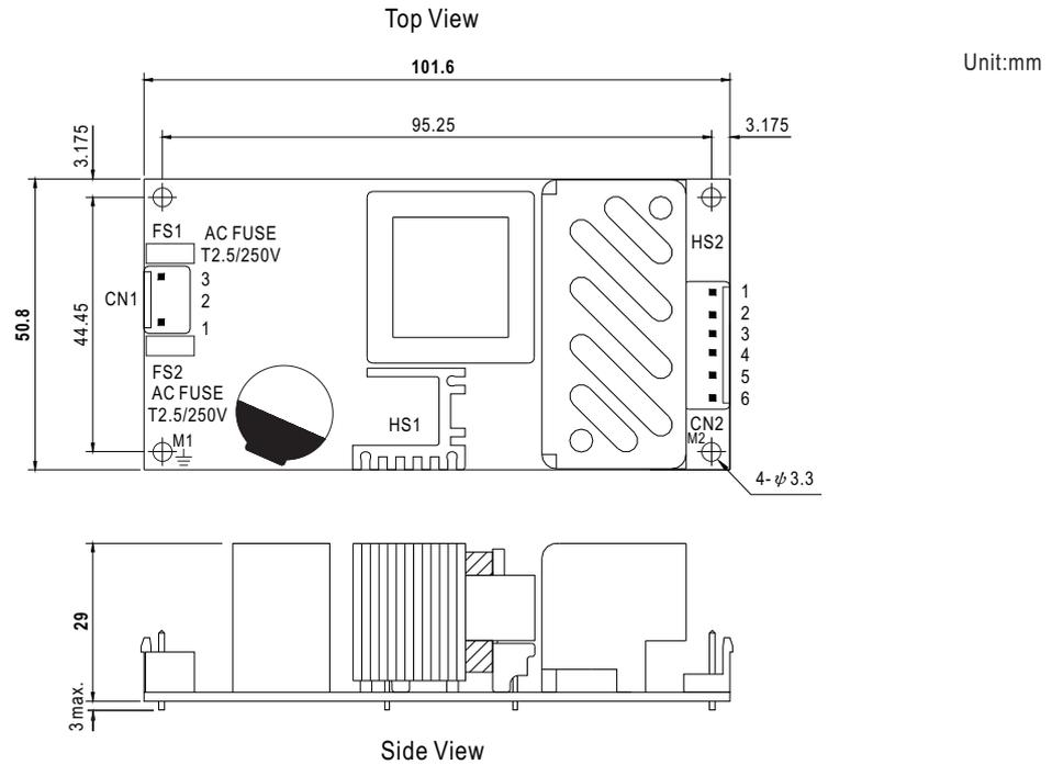
AC Input Connector (CN1) : JST B3P-VH or equivalent
