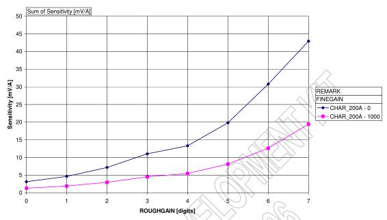
Adjustable sensitivity range from 2mV/A to 40mV/A
