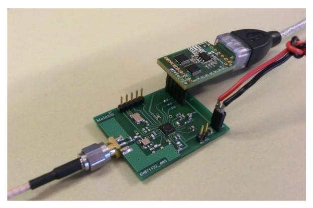
*Fig. 10:* How to connect the EVB71122 with the USB-SPI convertor
