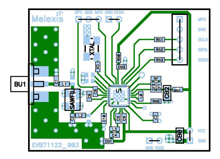
*Fig. 7: PCB Top-side view (averaging data slicer option)*
