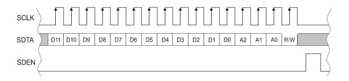
Fig. 6 Typical write sequence diagram
