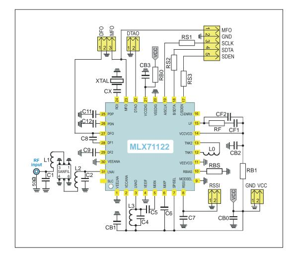
*Fig. 8: Application circuit for SPI Mode (peak detector option)*
