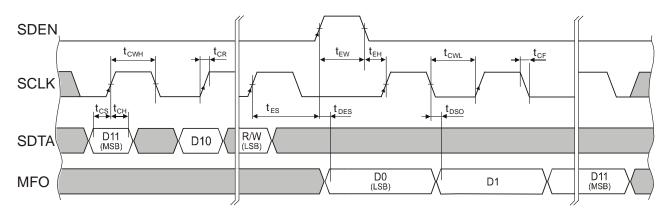
Fig. 8 SPI timing diagram
