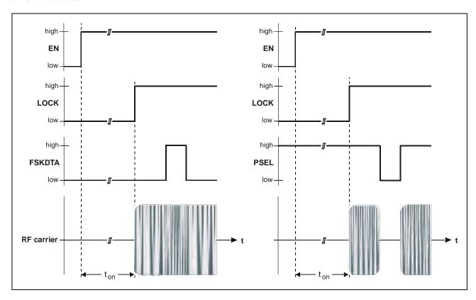
Fig. 5: Timing diagrams for FSK and ASK modulation
