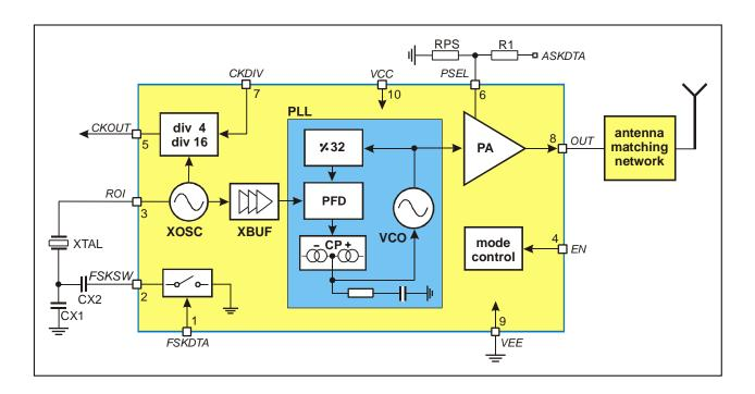
Fig. 1: Block diagram with external components
