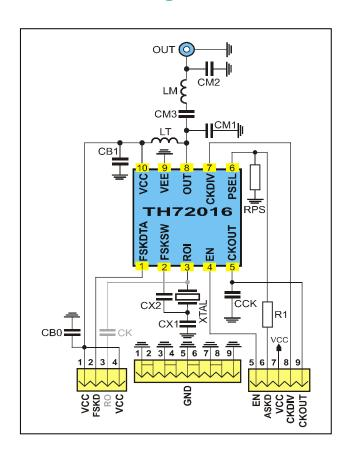
Fig. 6: Circuit diagram with 50  $\Omega$  matching network
