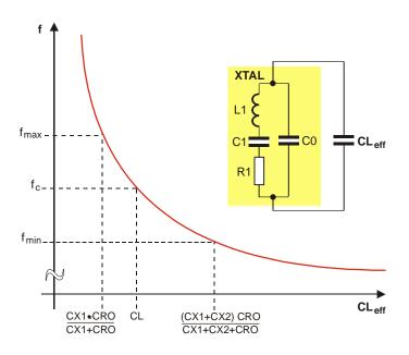
Fig. 3: Crystal pulling characteristic
