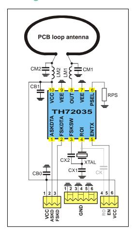
Fig. 6: Circuit diagram with loop antenna matching network
