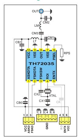
Fig. 7: Circuit diagram with 50  $\Omega$  matching network
