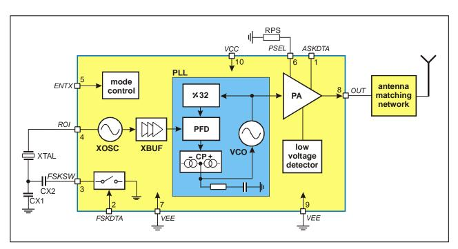
Fig. 1: Block diagram with external components
