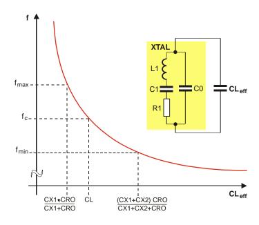
Fig. 3: Crystal pulling characteristic
