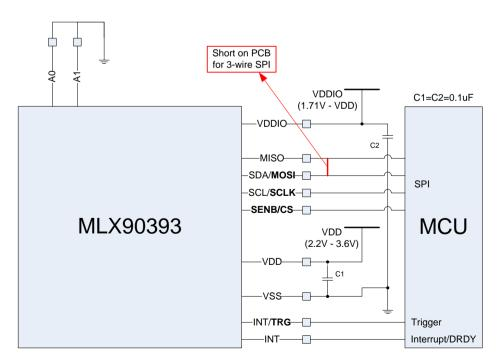
Figure 25: 3/4wire SPI recommended schematic
