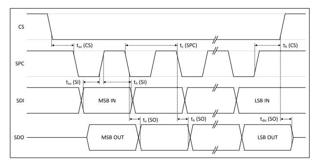
Figure 13: SPI Timing Diagram
