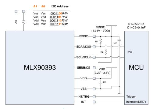
Figure 24: I<sup>2</sup>C recommended schematic
