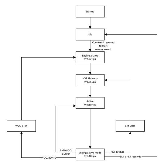
Figure 4: Top-level state diagram with indication of timings
