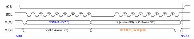
Figure 5: SPI communication example
