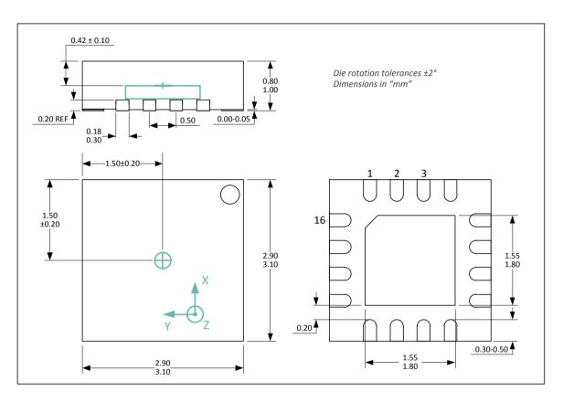
Figure 26: QFN-16 - Package Outline Drawing
