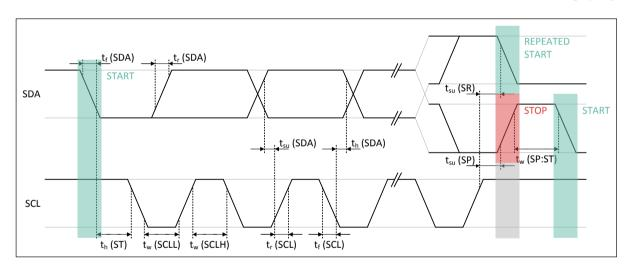
Figure 21: I<sup>2</sup>C Timing Diagram
