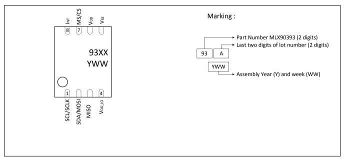
Figure 29: UTDFN-8 - Pinout and Marking
