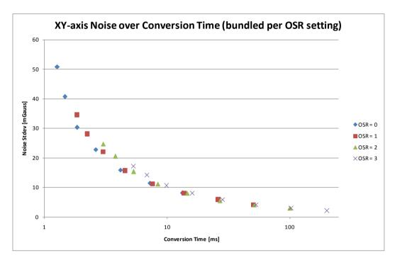
Figure 2: XY axis RMS noise versus conversion time, expressed in mGauss for GAIN SEL = 0x7
