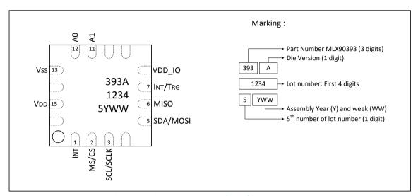
Figure 27: QFN-16 Pinout and Marking – Top view
