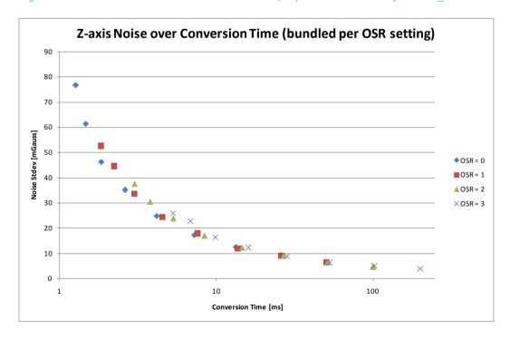
Figure 3: Z axis RMS noise versus conversion time, expressed in mGauss for GAIN\_SEL = 0x7
