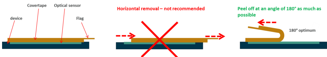
Figure 36: Grab the flag of the covertape and peel it off in an angle of 180° as much as possible.
