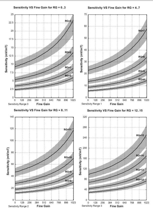
Figures 10.4-1...10.4-4 Sensitivity versus RG and FG. Important: You need option code 000 for Sensitivity Range 0 is option code 000, option code 1 for Sensitivity Range 1, option code 2 for Sensitivity Range 2 and option code 3 for Sensitivity Range 3.
