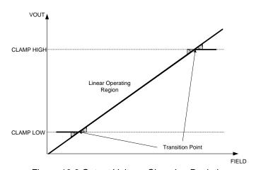
Figure 10.6 Output Voltage Clamping Deviation
