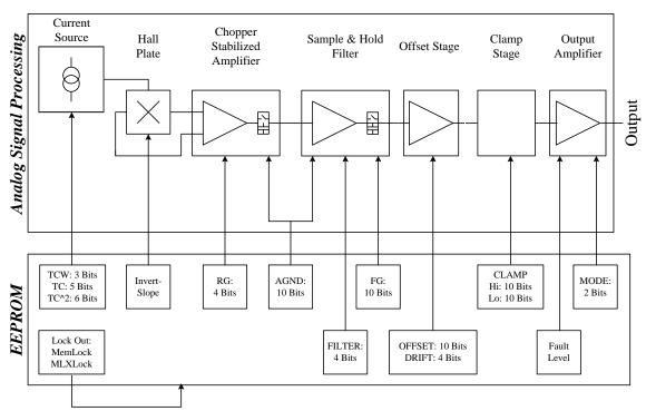
Figure 5-1 Detailed Block Diagram
