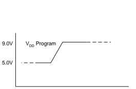
Figure 12.2-1 V<sub>DD</sub> Programming Level
