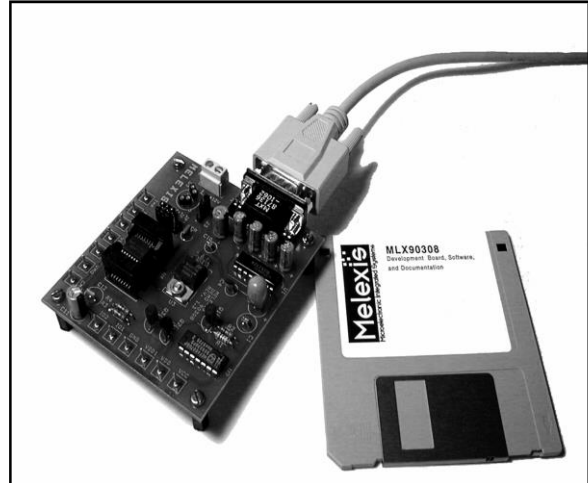
Figure 8. MLX90308 Evaluation Kit with MLX Software
