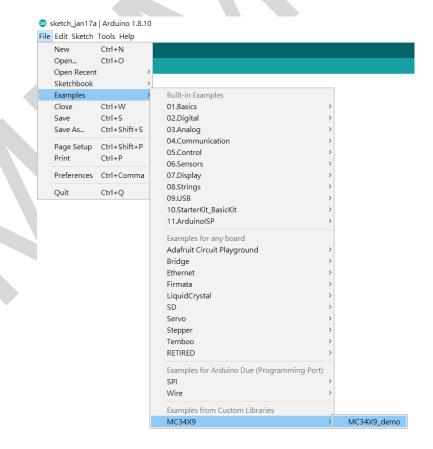
If you need the sensor running on SPI, please configure the bus as SPI in the MC34X9\_demo.ino shown as below. Otherwise, the default is I2C bus.
