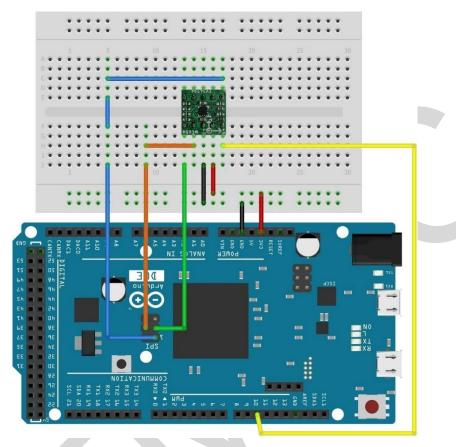
The EV3479A evaluation board can be easily wired to any microcontroller. This example shows a typical Arduino DUE platform. Please refer to the illustration below for connecting the related pins and then port the code to get the raw X, Y, Z sensor data.
