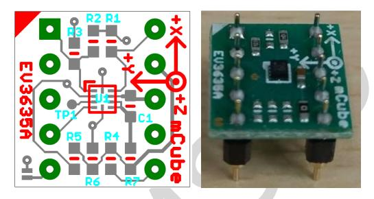
**R4, R5**: If using I2C and I2C pull-up resistors are needed for your application then install~4.7K $\Omega$  resistors into R4 (SCL clock pin) and R5 (SDA data pin) which are not installed by factory default. In addition, besides soldering resisters on R4/R5, you can add axial lead 4.7K ohm resistors to the SDA and SCL pin respectively. It will work the same either way.
