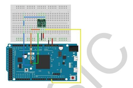
The EV3635A/B evaluation board can be easily wired to any microcontroller. This example shows a typical Arduino DUE platform. Please refer to the illustration below for connecting the related pins and then port the code to get the raw X, Y, Z sensor data.
