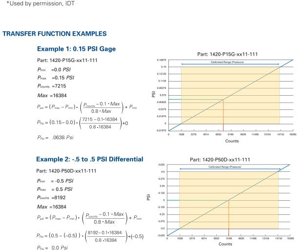
Communications to the 1420 is read only. To read the pressure counts, the master performs a read request by asserting a start condition, sending the 7 bit address of the part (If the part has an open address, 7 bits of anything is acceptable),
