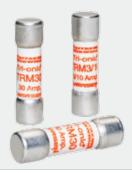
Tri-Onic® TRM time-delay midget fuses are rated 250 volts AC and are offered in ampere ratings from 1/10 to 30A. They have 12 seconds time-delay at 200% rating to provide supplemental protection of small motors, small transformers and other high inrush loads, plus many other 250 volt applications. (Not for Branch Circuit Protection).
