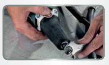
**Unparalleled productivity: Spindle stop** Lock the gearing by simply pressing a button and change the tool bit without needing a second key.
