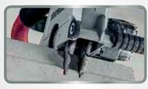
Widest range of applications Adjustable cutting depth 10 - 40 mm and cutting width 9 - 35 mm permits diverse applications with cutting disc Ø 125 mm.
