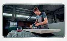
For coarse and fine sanding The SXE 450 TurboTec has a removable side handle for variable handle positions and an adjustable orbit diameter for coarse and fine finishing.
