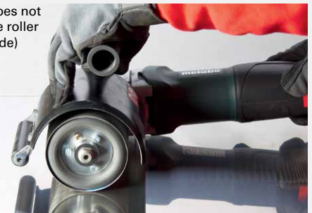
Preparation for mirror polishing: Metabo Burnishers with expansion roller, and Pyramid sanding belts from A160 (120 grit) to A6 (2000 grit).
