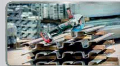
Cutting through 11 crash barriers Material: Sheet steel
