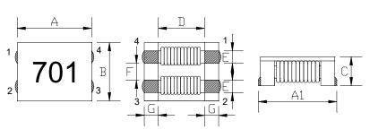
A: 9.0±0.5 mm A1: 9.5±0.5 mm B: 7.0±0.5 mm C: 4.8Max. mm D: 5.6Typ. mm E: 1.5±0.2 mm F: 2.0±0.2 mm G: 1.7±0.2 mm
