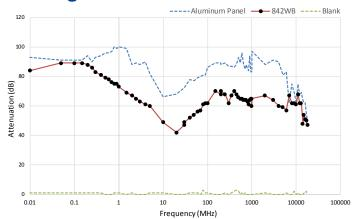
Test performed with a two-coat thickness.
