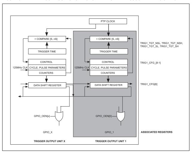
FIGURE 3-12: TRIGGER OUTPUT UNIT ORGANIZATION AND ASSOCIATED REGISTERS
