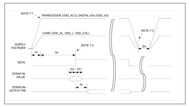
TABLE 7-5: RESET AND POWER SEQUENCE TIMING PARAMETERS (Note 7-1, Note 7-2, Note 7-3)
