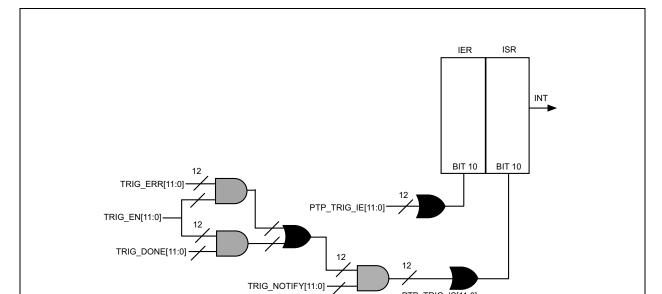
FIGURE 3-14: TRIGGER UNIT INTERRUPTS
