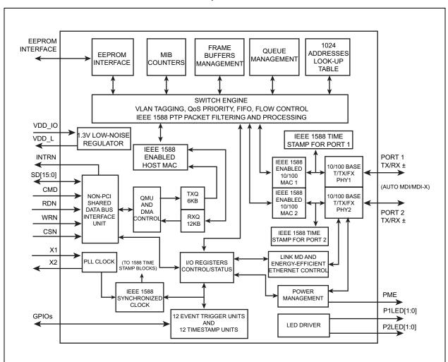
FIGURE 1-2: SYSTEM BLOCK DIAGRAM, KSZ8462HLI/FHLI
