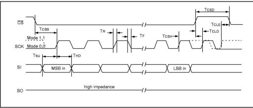
FIGURE 1-4: SERIAL OUTPUT TIMING
