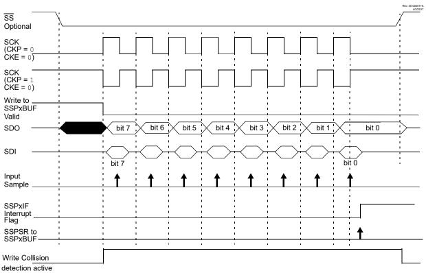
Figure 27-7. SPI Mode Waveform (Slave Mode with CKE = 0)
