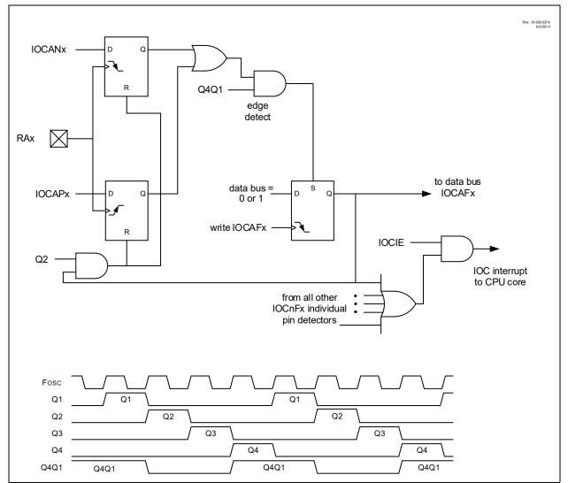
Figure 16-1. Interrupt-on-Change Block Diagram (PORTA Example)
