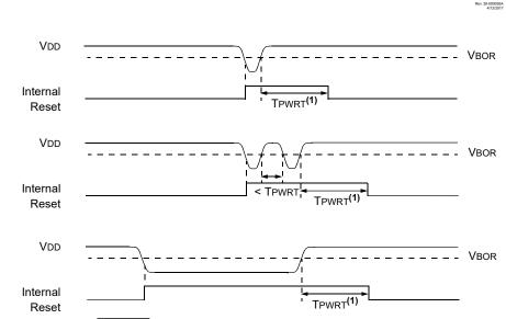
Note: T<sub>PWRT</sub> delay only if <u>PWRTE</u> bit is programmed to '0'.
