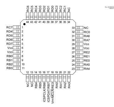
Figure 6. 44-pin QFN
