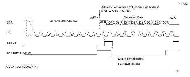
In 10-bit Address mode, the UA bit will not be set on the reception of the general call address. The slave will prepare to receive the second byte as data, just as it would in 7-bit mode.
