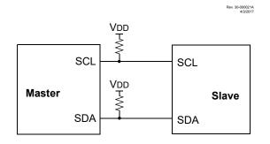
The I<sup>2</sup>C bus can operate with one or more master devices and one or more slave devices.
