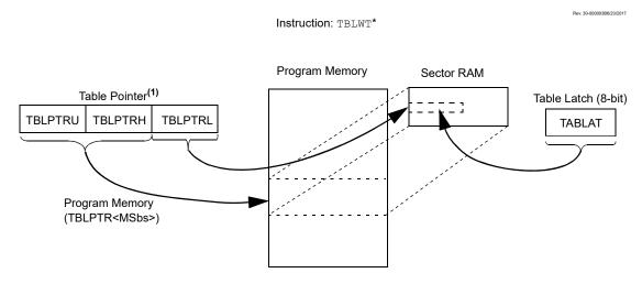
**Note** 1: During table writes the Table Pointer points to two areas. The LSbs of TBLPRTL point to an address within the sector RAM space. The MSbs of the Table Pointer determine where the sector will eventually be written.
