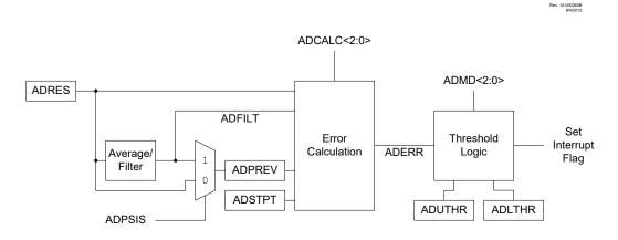
The operation of the ADC computational features is controlled by the 32.7.3.4 ADMD bits.
