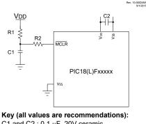
Key (all values are recommendations): C1 and C2 : 0.1  $\mu$ F, 20V ceramic R1: 10 k $\Omega$ R2: 100 $\Omega$  to 470 $\Omega$
