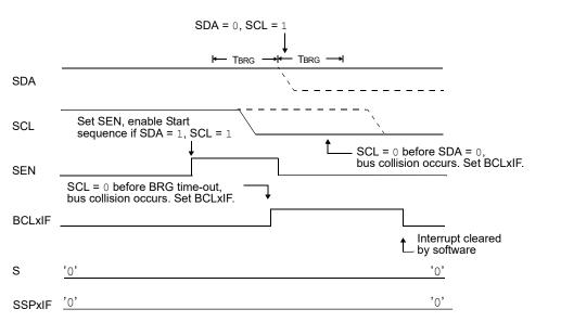
Rev. 30-000044A 4/3/2017 If the SDA pin is sampled low during this count, the BRG is reset and the SDA line is asserted early (Figure 27-35). If, however, a '1' is sampled on the SDA pin, the SDA pin is asserted low at the end of the BRG count. The Baud Rate Generator is then reloaded and counts down to zero; if the SCL pin is sampled as '0' during this time, a bus collision does not occur. At the end of the BRG count, the SCL pin is asserted low.
