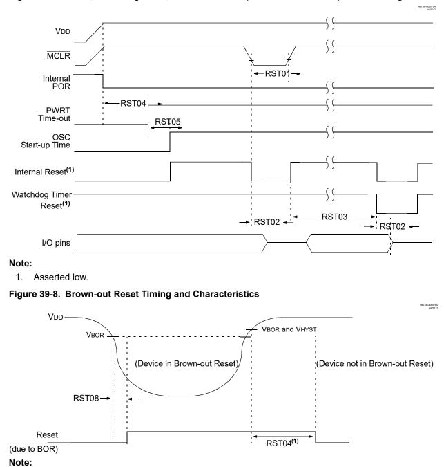
Figure 39-7. Reset, Watchdog Timer, Oscillator Start-up Timer and Power-up Timer Timing
