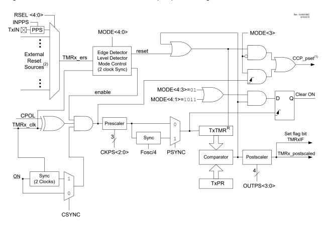
Figure 20-1. Timer2 with Hardware Limit Timer (HLT) Block Diagram
