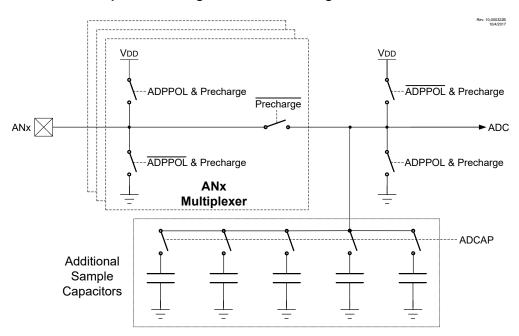
Figure 32-6. Hardware Capacitive Voltage Divider Block Diagram
