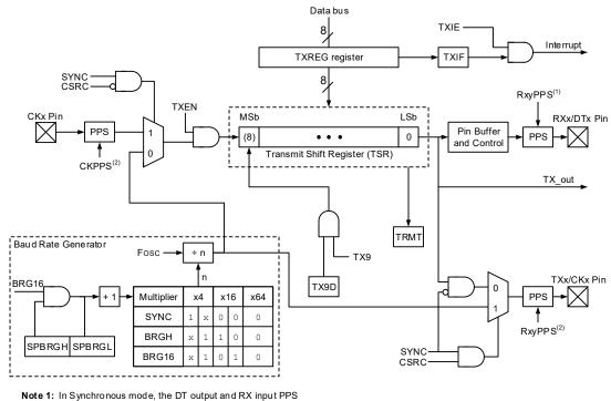
selections should enable the same pin. 2: In Master Synchronous mode the TX output and CK input
