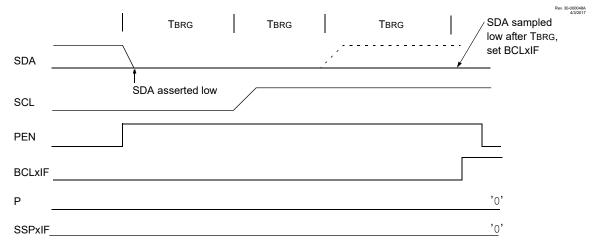
Figure 27-39. Bus Collision During a Stop Condition (Case 2)
