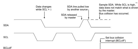
Figure 27-32. Bus Collision Timing for Transmit and Acknowledge
