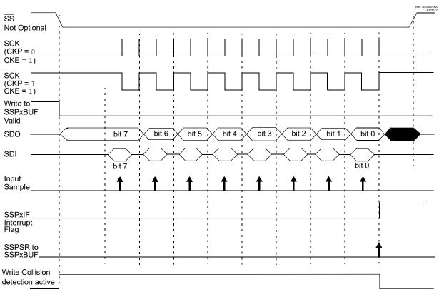
Figure 27-8. SPI Mode Waveform (Slave Mode with CKE = 1)
