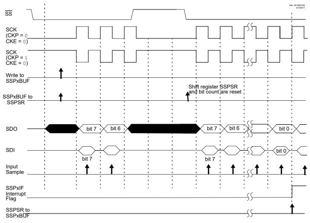
(MSSP) Master Synchronous Serial Port Module
