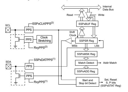
Note 1: SDA pin selections must be the same for input and output2: SCL pin selections must be the same for input and output
