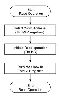
Example 11-1. Reading a Program Flash Memory Word MOVLW CODE ADDR UPPER ; Load TBLPTR with the base MOVWF TBLPTRU ; address of the word CODE ADDR\_HIGH MOVLW MOVWF TBLPTRH MOVLW CODE ADDR LOW MOVWF TBLPTRL READ WORD:
