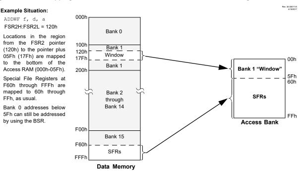
Remapping of the Access Bank applies only to operations using the Indexed Literal Offset mode. Operations that use the BSR (Access RAM bit is '1') will continue to use direct addressing as before.
