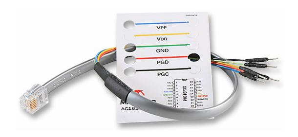
This cable breaks out the ICD 2 RJ-11 to male pins for plugging into a solderless breadboard.
