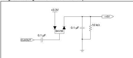
Most bus switches have extremely low-current requirements, so despite the limited current sourcing capability of CLKOUT, it can potentially be used to both generate ~5V required for the bus switches and still be used as a clock source for other circuitry in the application.
