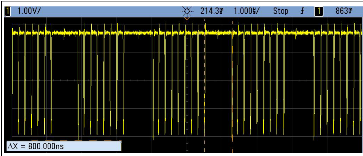
FIGURE 9: putpixel TIMING DIAGRAM
