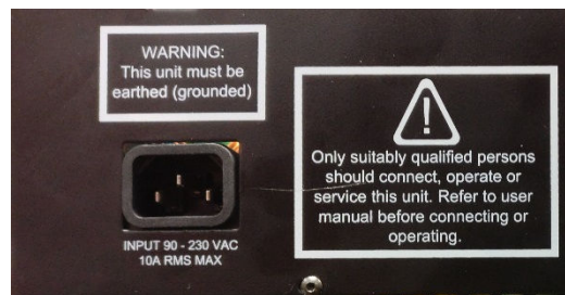
Figure 2-2. dsPICDEM MCHV-3 Development Board AC Mains Interface
