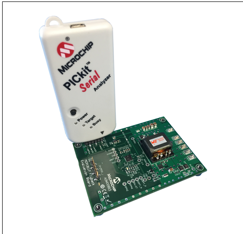
FIGURE 3-1: PICKit Serial Analyzer Connection to the Board.
