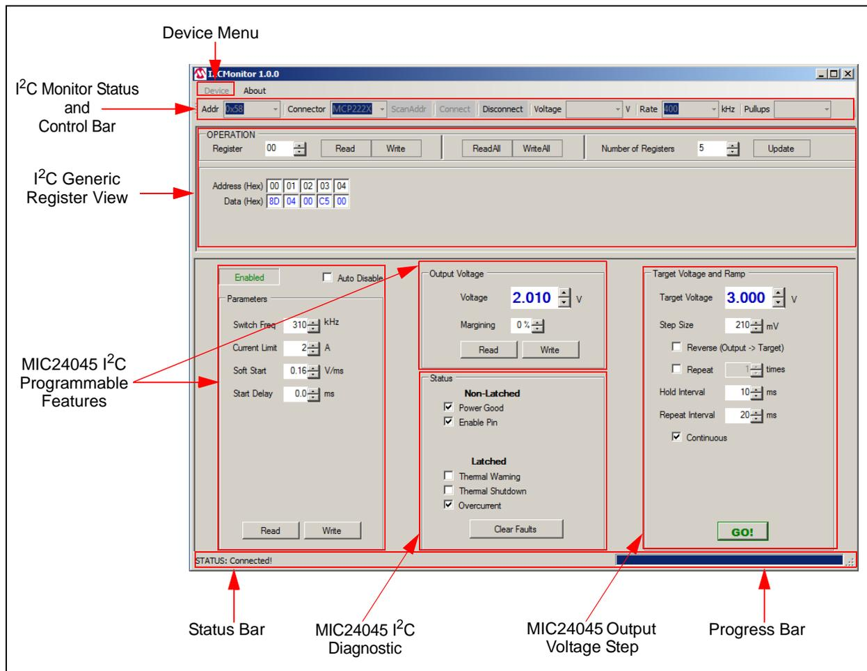
**FIGURE 4-1:** I<sup>2</sup>C Monitor Graphical User Interface Main Window - MIC24045 View.
