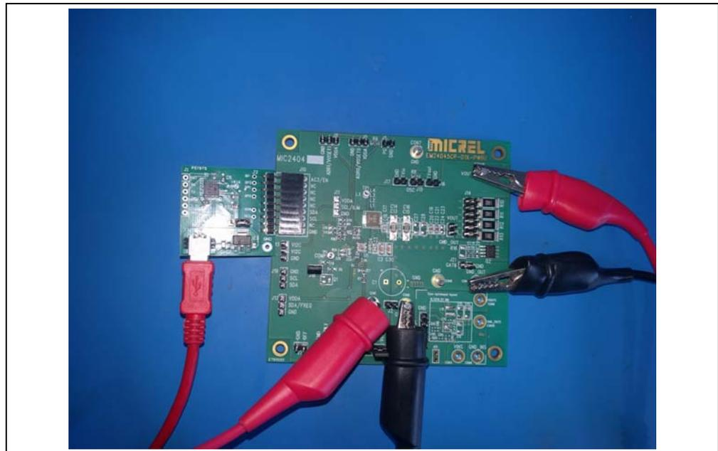
**FIGURE 2-1:** MIC24045 with MCP2221 Board Connection.
