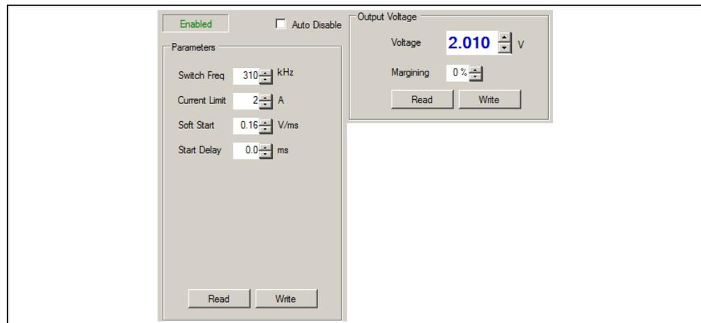
**FIGURE 4-4:** MIC24045 I<sup>2</sup>C Programmable Features Area.
