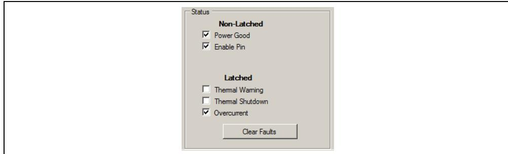
**FIGURE 4-5:** MIC24045 I<sup>2</sup>C Diagnostic Area.
