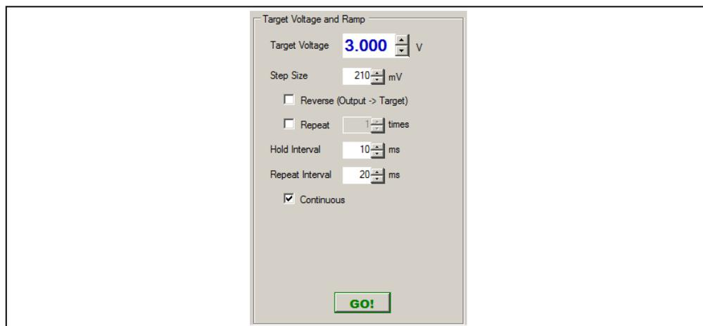
**FIGURE 4-6:** MIC24045 Output Voltage Ramp Area.
