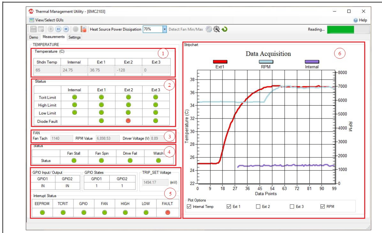
FIGURE 3-14: Temperature Sensor View – Measurements Tab.
