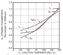
Figure 6. Dynamic Parameters vs. Junction Temperature
