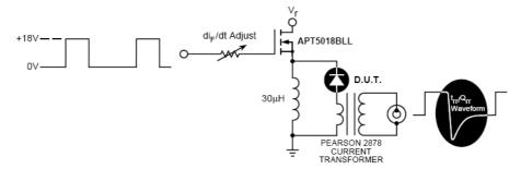
Figure 9. Diode Test Circuit
