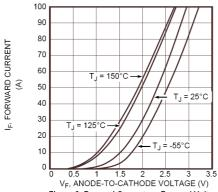
Figure 2. Forward Current vs. Forward Voltage
