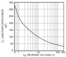
Figure 8. Junction Capacitance vs. Reverse Voltage
