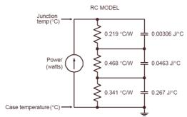
FIGURE 1b, TRANSIENT THERMAL IMPEDANCE MODEL
