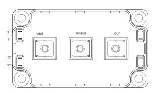
$$\begin{split} V_{DSS} &= 1000 V \\ R_{DSon} &= 130 m \Omega \text{ typ } @ \text{ Tj} = 25^{\circ} \text{C} \\ I_D &= 65 \text{A} @ \text{ Tc} = 25^{\circ} \text{C} \end{split}$$
