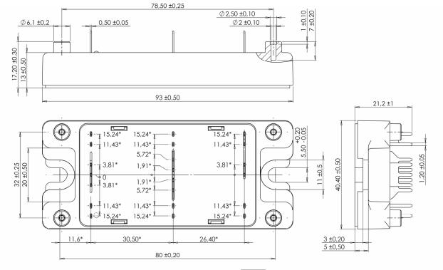
ALL DIMENSIONS MARKED "\*" ARE TOLERANCED AS : + Ø 1
