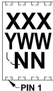
8-Lead TDFN (2x3x0.75 mm)
